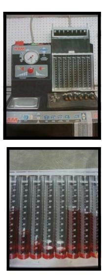
From above left ,our guest speaker Stan " The Man" from San Diego Carburetor/ Fuel injection shop with pictures of the machine used to test/tune fuel injectors notice the different flow rates of the injectors as tested and the different volumes of fluid collected demonstrating the variation in flow rate of the injectors ,wich affects the performance of your car. Bellow pictures of the General Meeting attendance and some of the cars in the parking lot.
